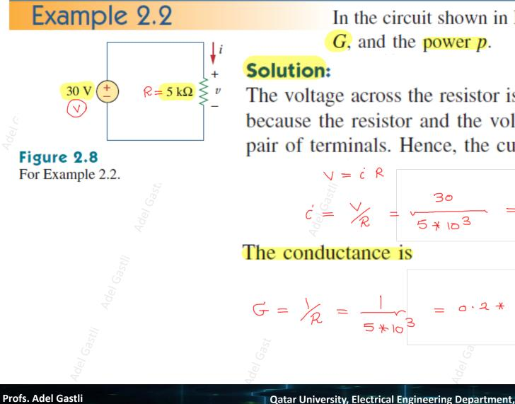
In the circuit shown in Fig. 2.8, calculate the current *i*, the conductance G, and the power p.
