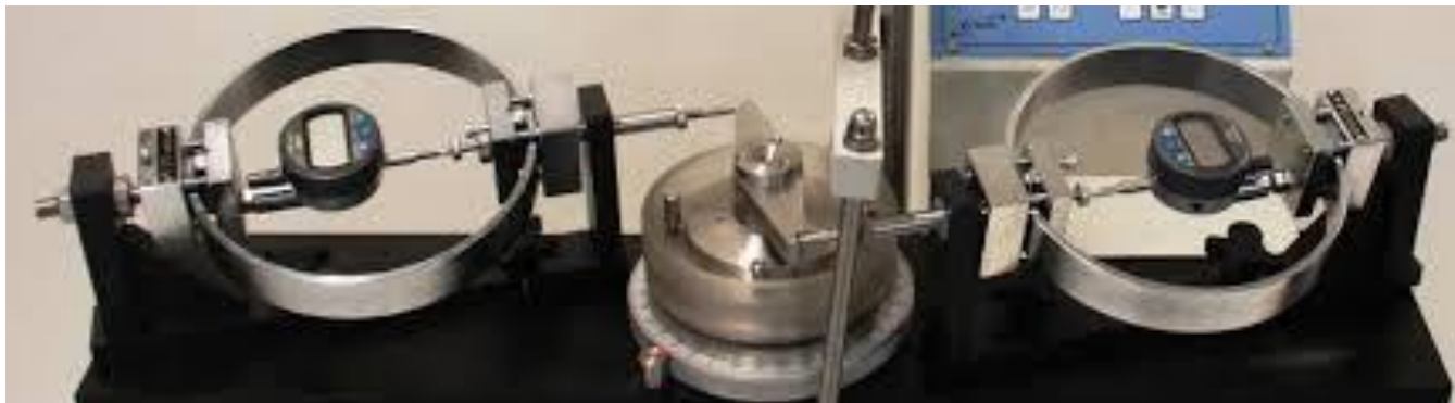
Torque arm held in place by two proving rings in torsional ring-shear apparatus
