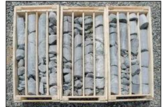
Rock borehole cores
