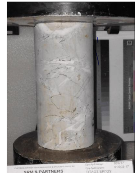
Rock specimen ready for unconfined compression test
