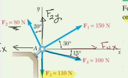
Four forces act on bolt A as shown. Determine the resultant of the forces on the bolt.
